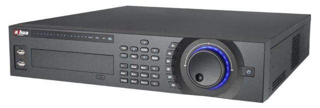
**DH-DVR0404LF-S:** Full channel 2CIF or 2ch@D1+2ch@CIF realtime recording; 4 channel video inputs and 4 channel audio input; 4 channel loop outputs and 1 channel spot output. It can support HDMI, VGA, TV, USB2.0 and 4HDD.
